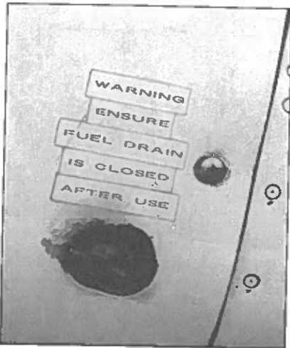
Engine fuel strainer with warning sign.
